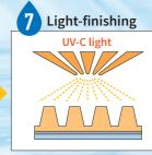
Expose to UV-C light to eliminate a plate tackiness.
