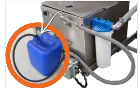
Liquid filling & emptying system
