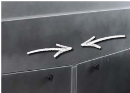
Inclination of tub for less liquid carry-over
